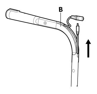
7. Connect the cable jack with the DC socket, then secure the cable with the Extension cover (C).
