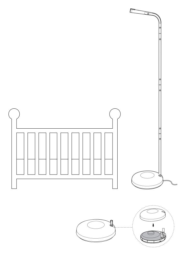
Install the Baby Unit onto the First extension (A). Connect the adapter to the end of the cable and the power supply to power up the Baby Unit. Slide the switch to **ON** to power your Baby Unit on.
