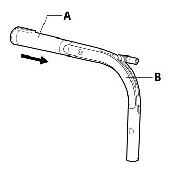
3. Pick one pole and pass the cable jack through the pole, then connect the pole with the Base.
